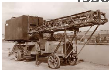
A CR20 vehicle-mounted crane, designed by Haulotte.
