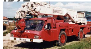
GB18 Haulotte, first «City crane» in the world - high travel speed, quick setting up and lifting cabin.
