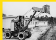
The SK2 compact shovel - the world's first tyre-mounted compact shovel with tailswing.
